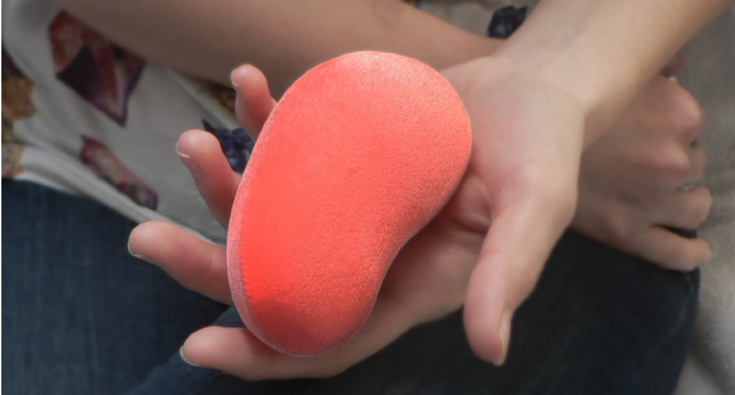
Fig. 1. The breathing friend helps to relief stress by lowering the user's breathing frequency.
