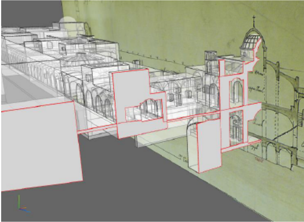
Fig. 1. Digital reconstruction of historical architectural drawings. A good documentation is needed to retrace from which origin the reconstruction has been developed.
